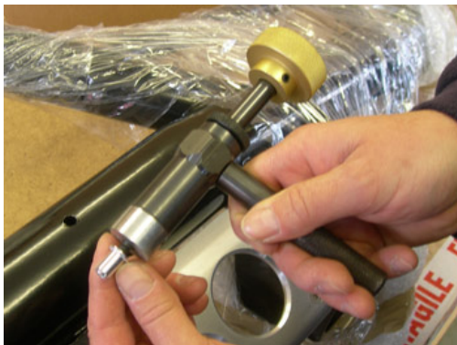
4) Fit the riv nut onto the setting tool and set.
