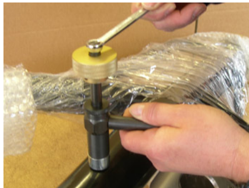
4) Fit the riv nut onto the setting tool and set.
